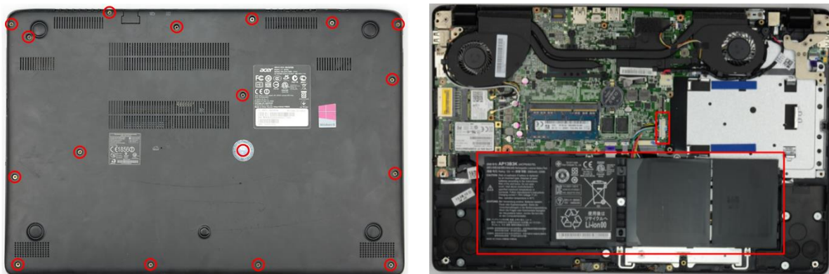
Figure 4: Opening of the housing to remove the integrated notebook battery from DUT_2
