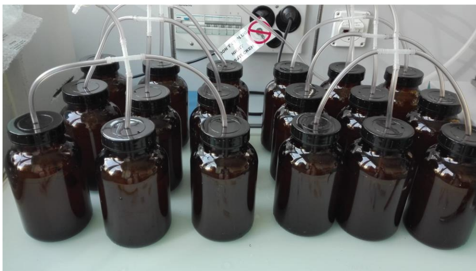
Figure A 3: Experimental setup of OECD 308-type studies
