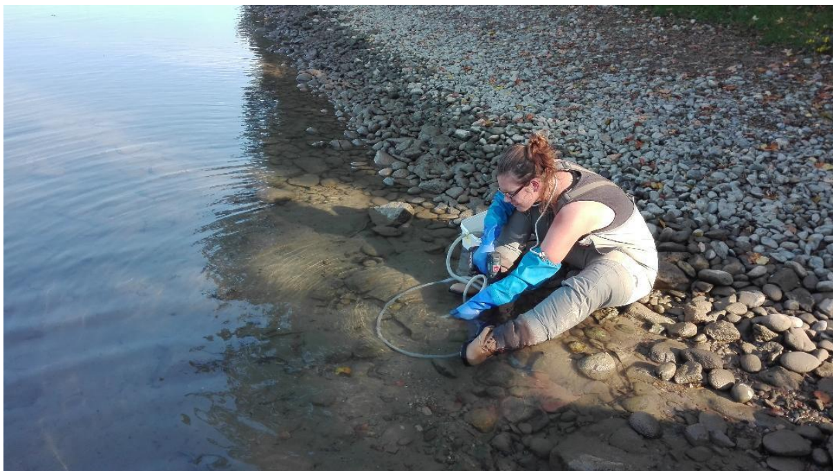
Figure A 1: Sampling of sediment from the Rhine for OECD 309-type suspension tests
