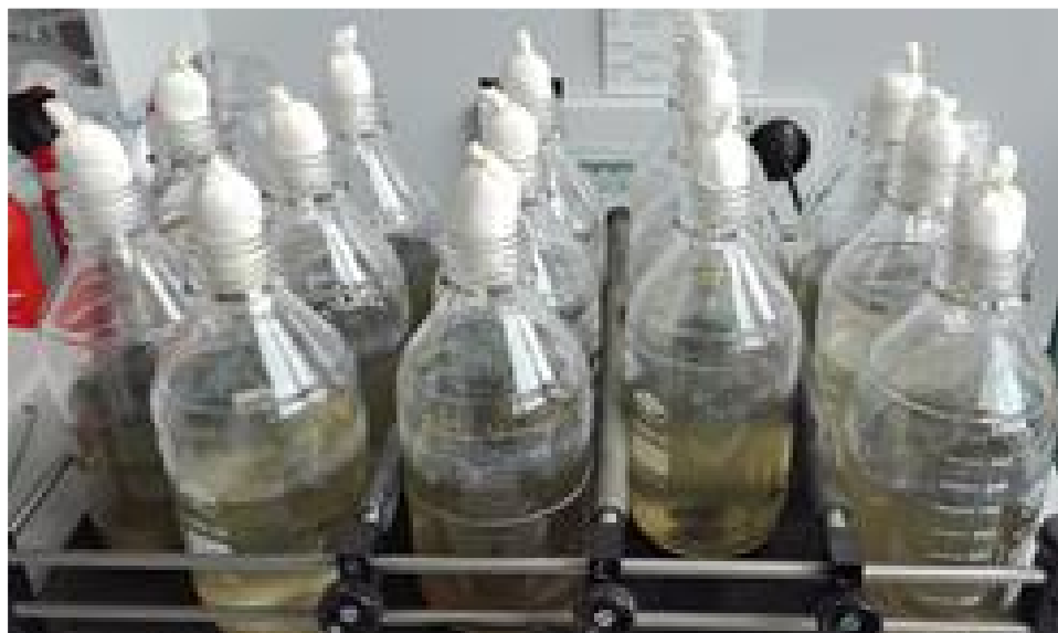
Figure A 2: Experimental setup of OECD 309-type suspension tests
