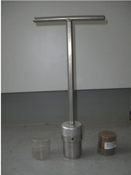
Figure 16 Soil corer with plastic cartridges (l: empty r: filled) used for sampling of microarthropods and enchytraeids.
