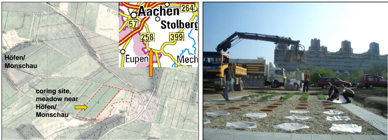
Figure 6 left: Location of the coring site of TMEs in Höfen / Monschau (North Rhine Westphalia). No. 4 Intensive meadow (Coring Site), No. 5 adjacent Extensive Meadow involved in pre-screening of soil organisms; right: Placing of TMEs into the test facility
