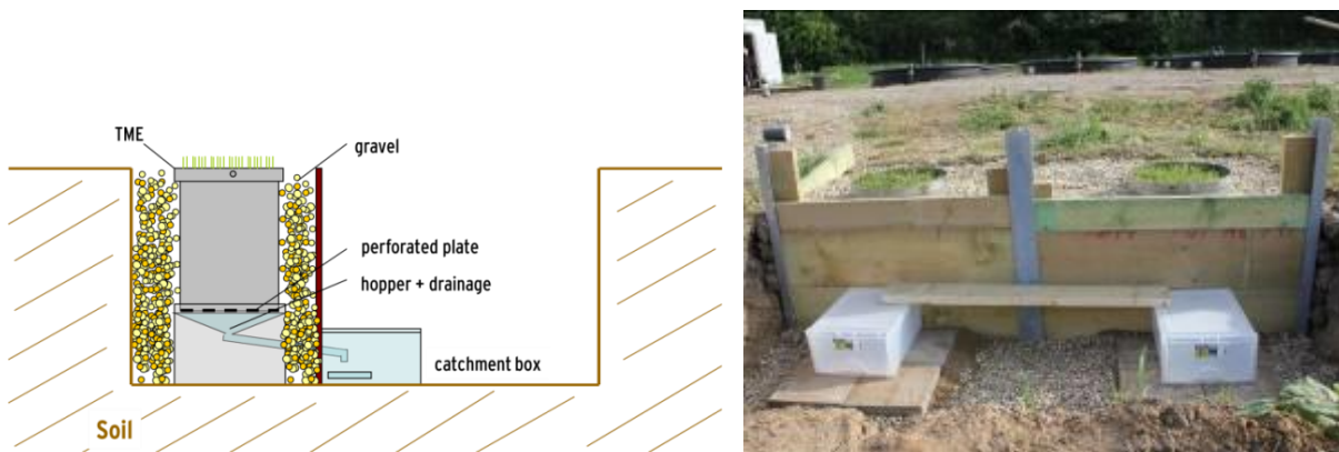
Figure 18 Schematic profile (left) and picture of the facility for measurement of leachate water (right)
