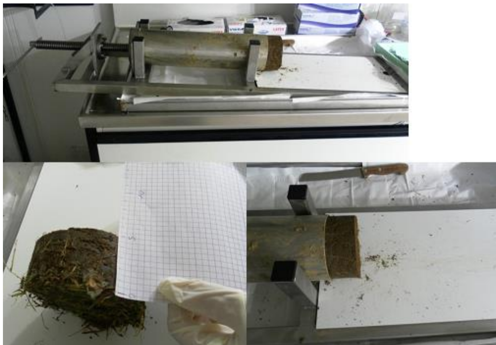
Figure 15 The soil core was pushed out of the column through the bottom and cut into subsamples.
