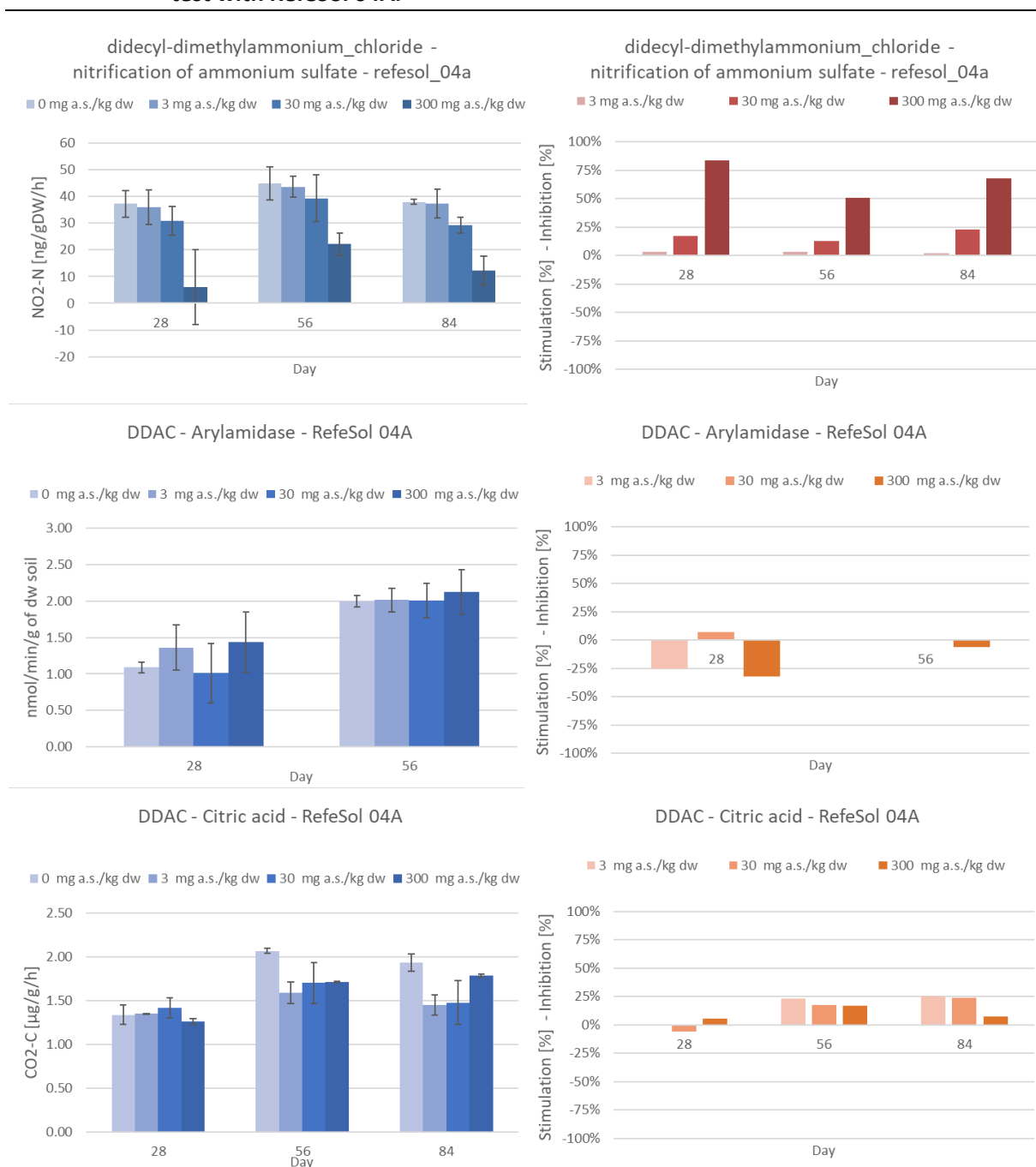
Figure 67: Exemplary results of the potential nitrification (ISO 15685; upper figure), the exoenzymatic activity (ISO 20130; mid figure) and the SIR with citric acid (MicroResp™) for DDAC at application rates of 3, 30 and 300 mg/kg dw soil in the test with RefeSol 04A.
