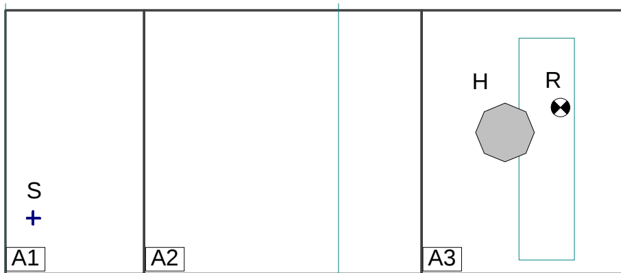
Figure 5.3.14-1: Octagonal house H on ground with different heights and acoustic properties (S source, R place of immission, A1 area with G=0.5, A2 area with G=0.9, A3 area with G=0.2) (Source: Umweltbundesamt [9])
