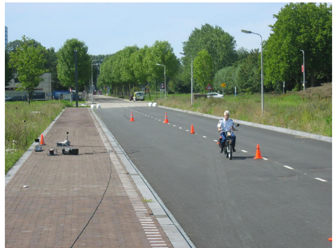
Motorcycle Pass By test
