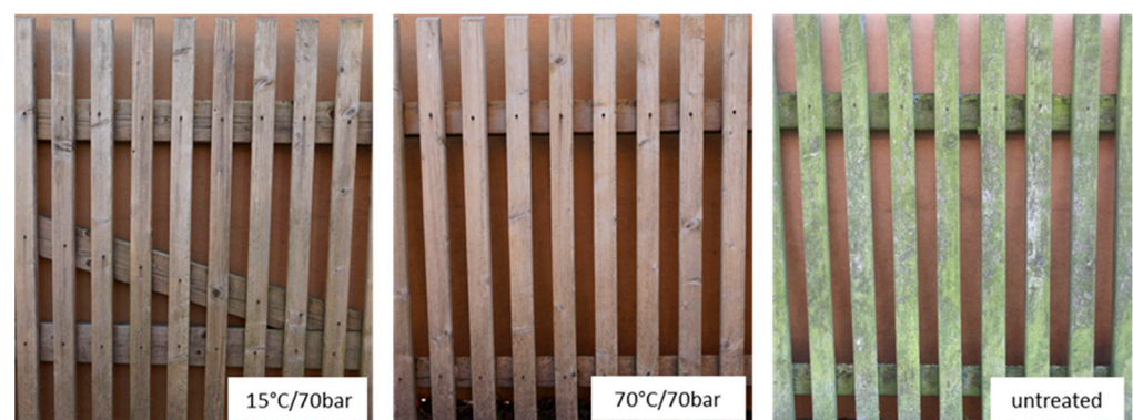
Figure 5. Examples of the fence panels with different treatments after six months.
