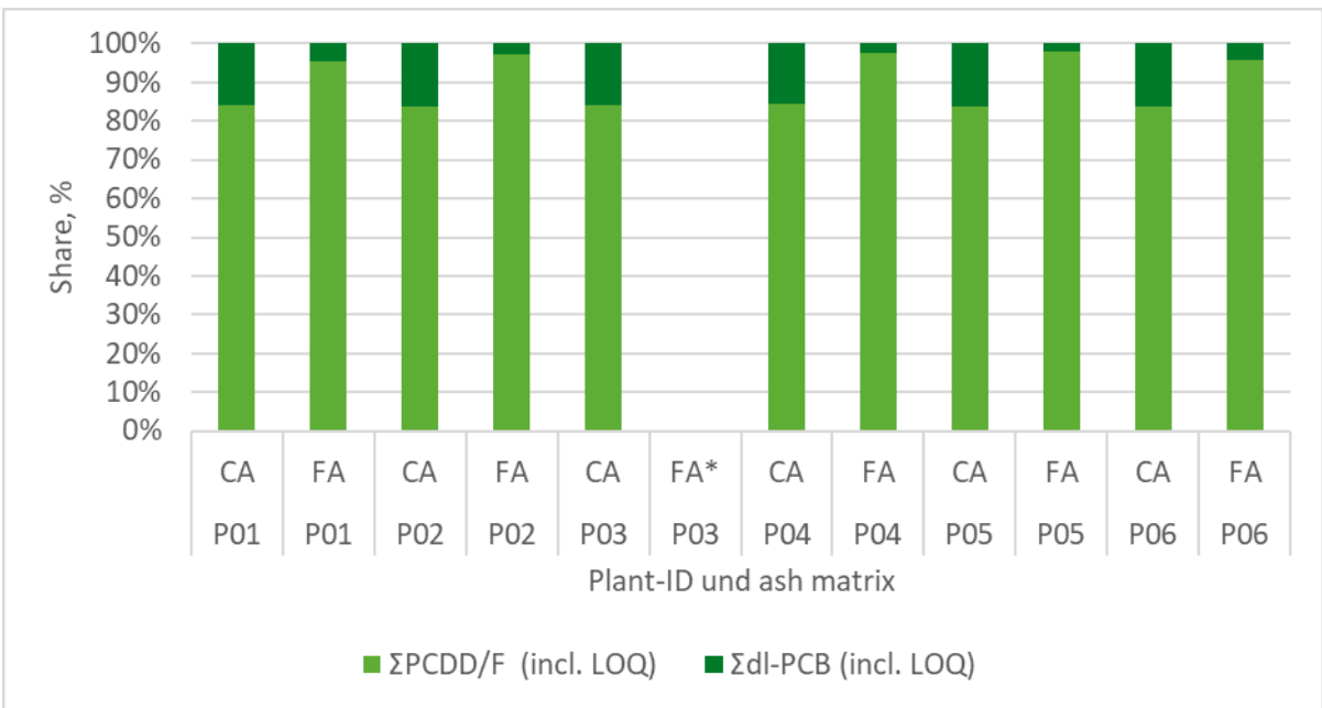
Figure 10: Contribution of PCDD/Fs and dl-PCBs to total TEQ in ash from single-chamber combustion plants.
