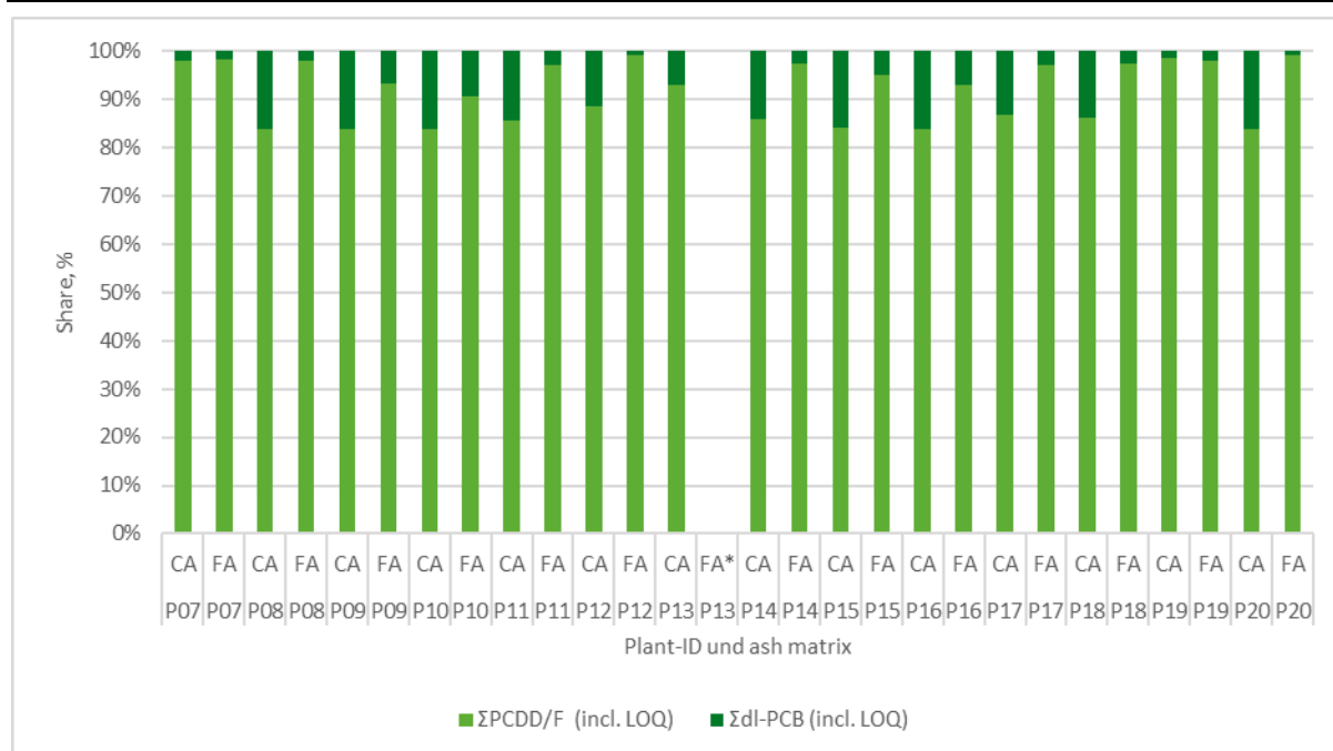
Figure 13: Contribution of PCDD/Fs and dl-PCBs to total TEQ in ash from solid fuel boilers.
