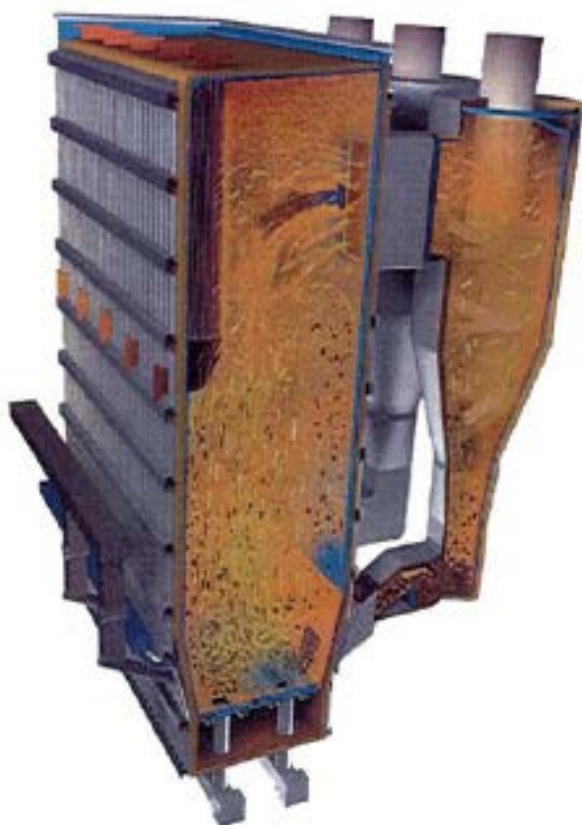
Figure BM 6: Fuel and bed material flow in a biomass fired CFB boiler
