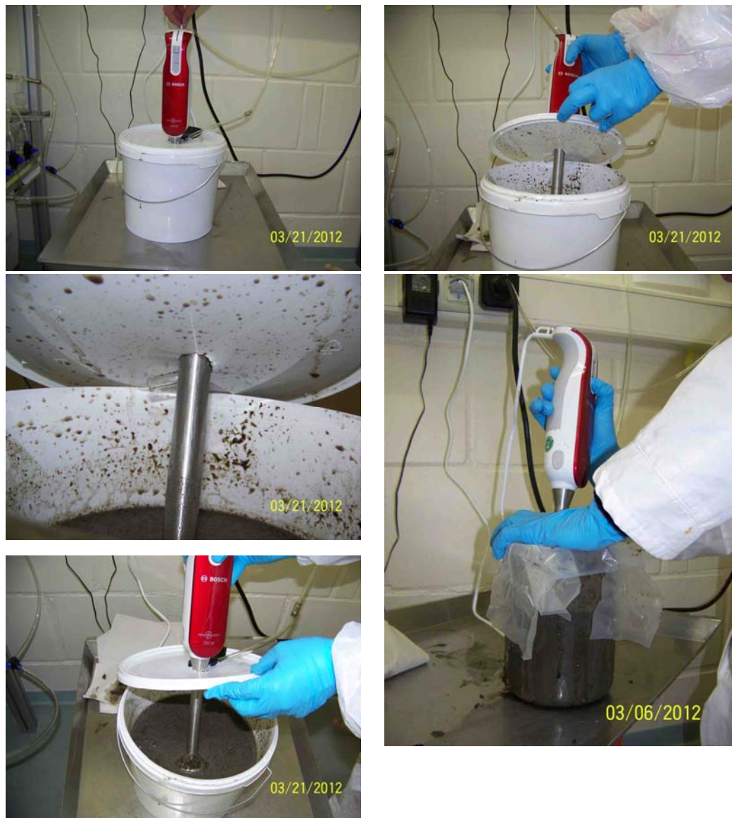
Figure 9: manure homogenization procedure while keeping anaerobic conditions
