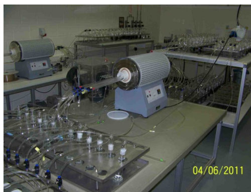
Figure 11: tube furnaces for combustion of methane to carbon dioxide and subsequent trapping in NaOH-solution
