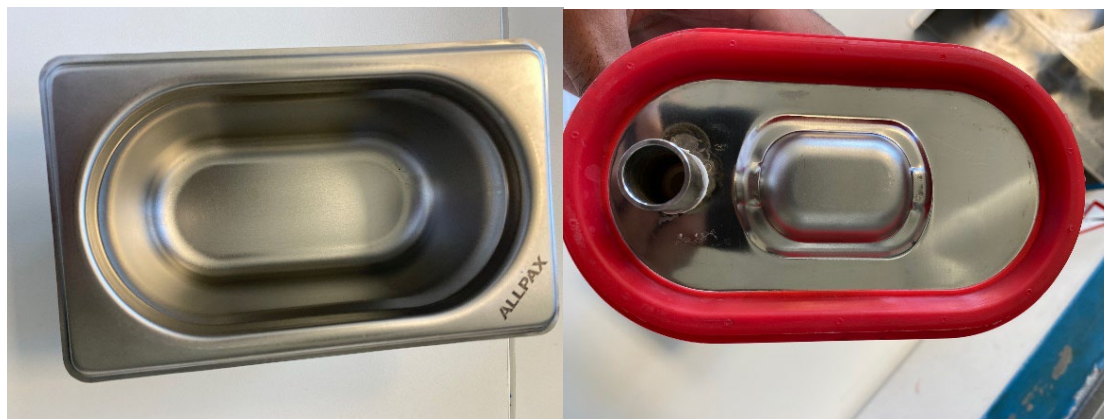
Figure 5: Vessel (left) and top cover (right) used for laboratory simulations on hard surfaces
